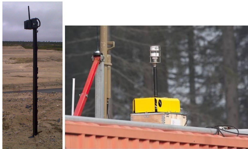
Figure 8. Chemical sensor (left), EMAS weather station (right)
